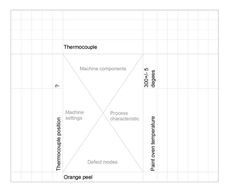
The matrix begins by starting with the defect mode from the QA matrix. Then working anticlockwise the team review the critical process characteristics, in this example the temperature of the paint oven. However at the time the defect occurred, the process control records showed that the paint oven was within the defined tolerance.
